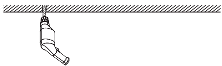
1. Drill a \varnothing 6\text{mm} hole
